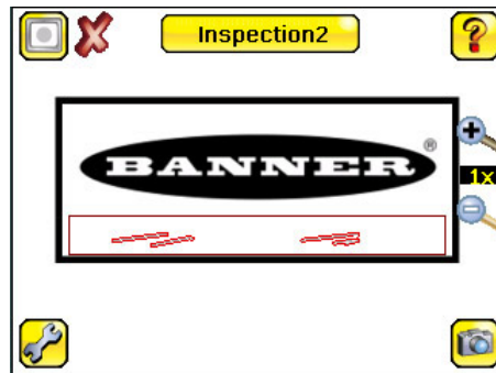
Figure 101. Blemishes Found During the Inspection
