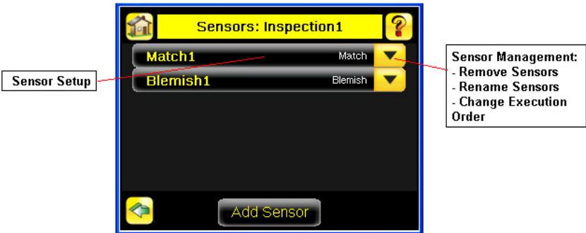
Figure 130. The New Sensor is Added to the Inspection
